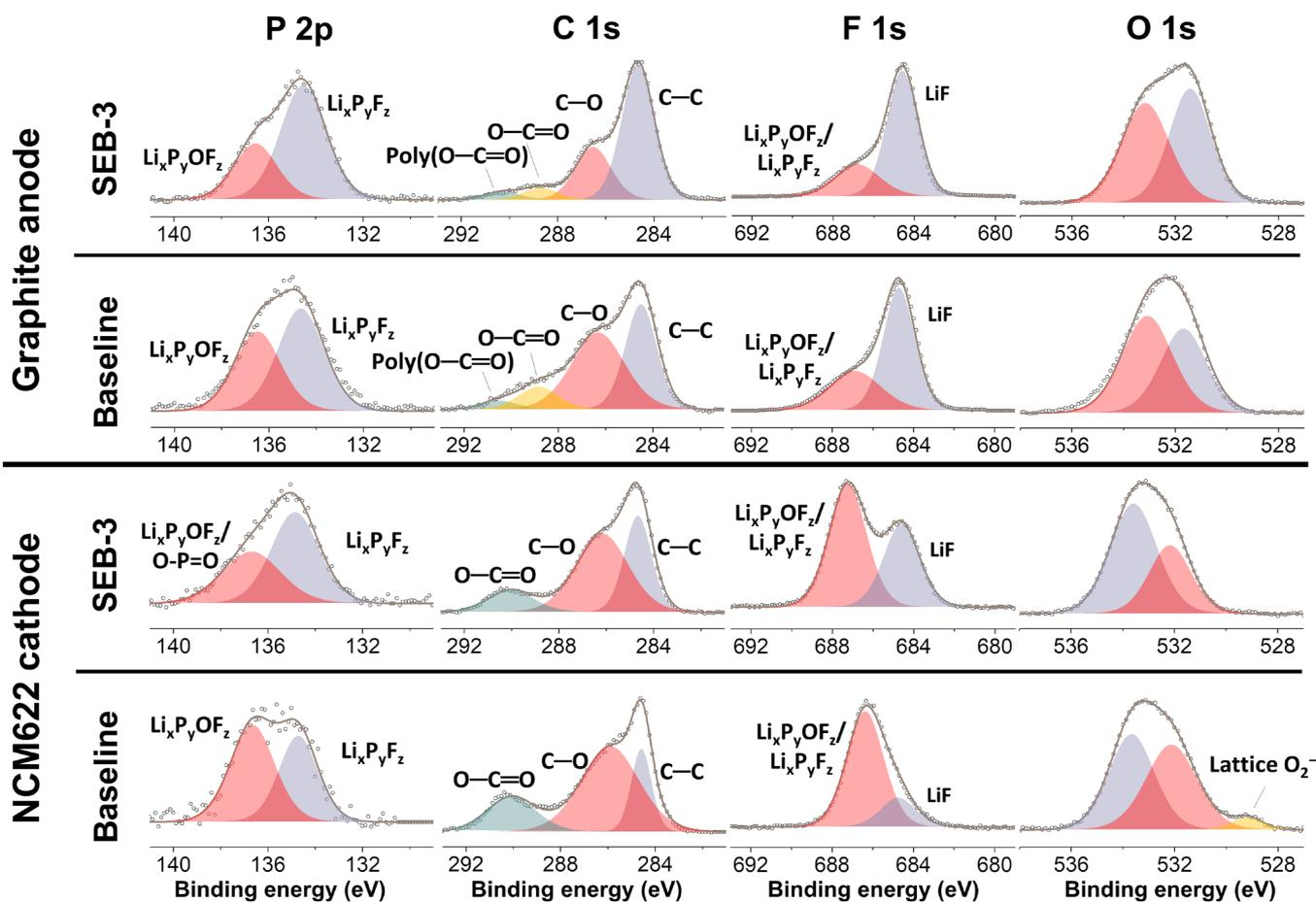
**Fig. 6.** XPS core spectra comparison for aged baseline and SEB-3 electrodes. The graphite and NCM622 electrodes are taken from the baseline cell after 956 cycles and the SEB-3 cell after 4021 cycles.
