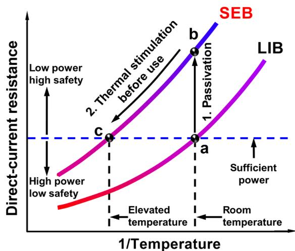
**Fig. 1. Principles and advantages of a SEB versus a conventional LIB.** DCR is shown to vary with the inverse of temperature for both batteries, where the upper curve for the passivated SEB is always safer due to higher DCR. The SEB can, however, achieve a similar power output to the LIB by thermal stimulation before operation, shown as going from point b to c.
