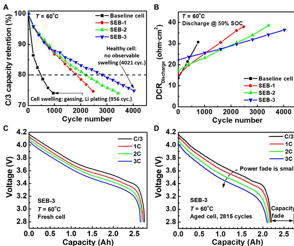
**Fig. 4. Comparison of cycling stability at 60°C.** (A and B) Capacity retention and DCR of the SEB cells versus the baseline LIB cell during cycling at 60°C. The cells are charged with CCCV protocol at 1 C to 4.2 V with a cutoff current of C/20 and then discharged at 1 C to 2.8 V. (C and D) Discharge curves of the fresh SEB cell versus aged cell.
