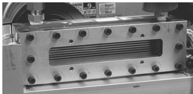
Figure 1. Experimental setup of the transparent fuel cell with an active area of 14 \text{ cm}^2 and seven parallel flow channels on both anode and cathode.
